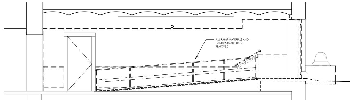
4 DEMOLITION SECTION - BASEMENT EAST ACCESSIBLE ENTRANCE, LOOKING NORTH AT RAMP RAILING
