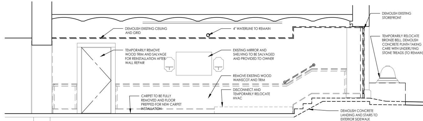
5 DEMOLITION SECTION - BASEMENT EAST ACCESSIBLE ENTRANCE, VIEW LOOKING NORTH AT NORTH ELEVATION
