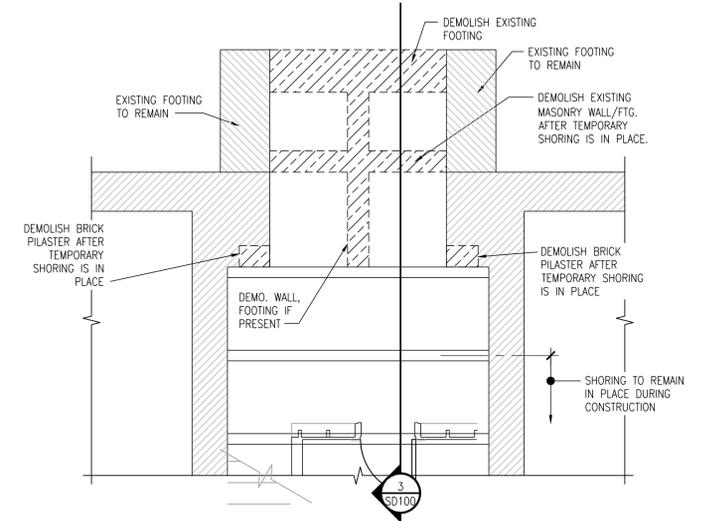
**2 WEST STAIR BASEMENT LEVEL DEMOLITION PLAN**
