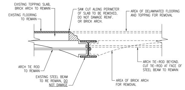
**4 DEMO DETAIL AT EXISTING STEEL BEAM**
